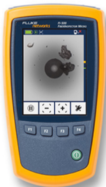
FI-500 displaying a dirty fiber endface
